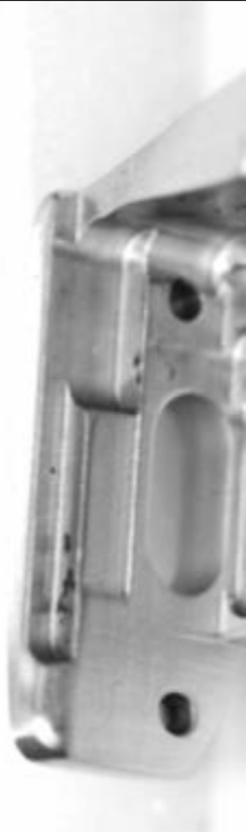
Fine blanking before hardening
