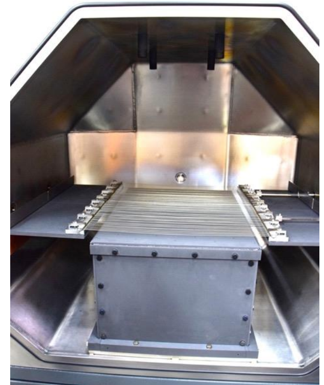
Graphite box to adjust filament-tool spacing
