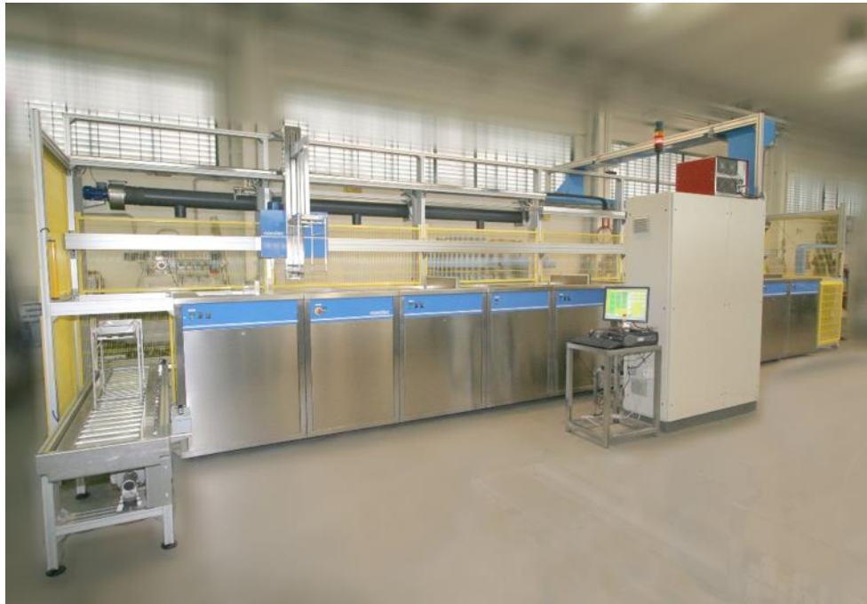
Multi-tank wetbench with automated handling
