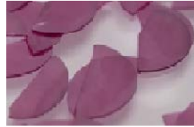
Half moon wafer sawing with calibrated thickness
